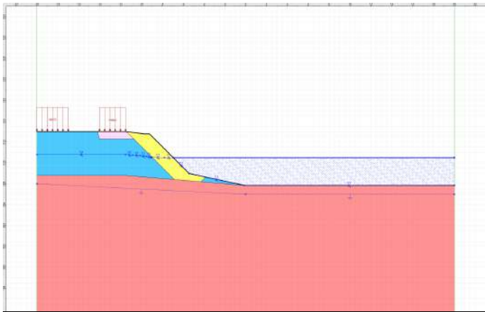
Phase 10: Enrochements 1H/1V eh=2.0m
