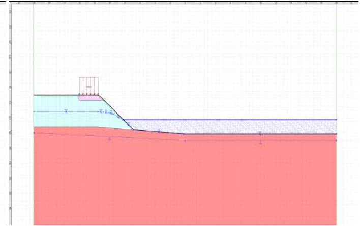
Phase 3: Talus provisoire 1H/1V Bief 209.75 NGF + surcharge
