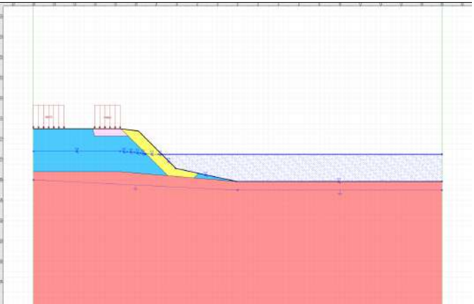
Phase 9: Enrochements 1H/1V eh=1.5m
